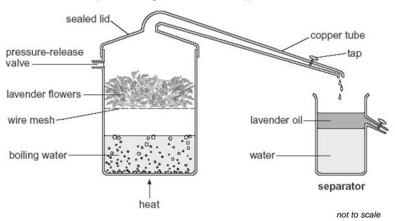
Water vapour and lavender oil vapour pass down a copper tube towards a separator.
