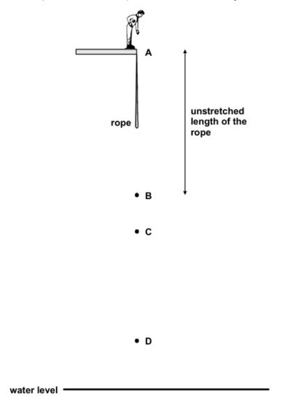
The man falls past B, and the rope begins to stretch. He falls past point C to point D, which is the lowest point he reaches. Then he begins to move upwards again. Eventually he comes to rest at point C.
