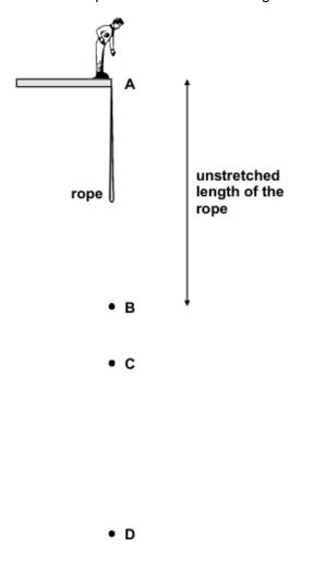
The man falls past B, and the rope begins to stretch. He falls past point C to point D, which is the lowest point he reaches. Then he begins to move upwards again. Eventually he comes to rest at point C.
