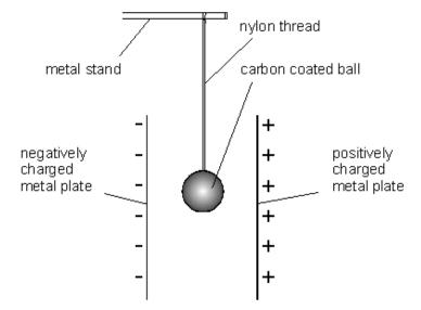
The plates are charged. The ball is moved across to touch the positive plate, and becomes positively charged. It is repelled from the plate.
