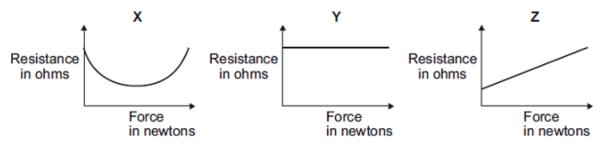
Which of the sensors, X, Y or Z, would be the best one to use as a force sensor?
