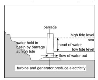
Gates in the barrage are open when the tide is coming in and the basin is filling to the high tide level. The gates are then closed as the tide begins to fall.
