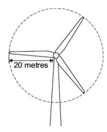
(a) The blades of the turbine are 20 metres long. On average, 15 000 kg of air, moving at a speed of 12 m/s, hit the blades every second.
