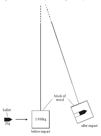
A bullet is fired into a block of wood suspended by a long thread.
