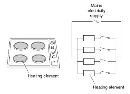
When all four heating elements are switched on at full power the hob draws a current of 26 A from the 230 V mains electricity supply.
