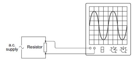
Each horizontal division on the oscilloscope screen represents a time of 0.01s.
