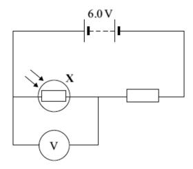
(a) The graph, supplied by the manufacturer, shows how the resistance of the component labelled **X** varies with light intensity.
