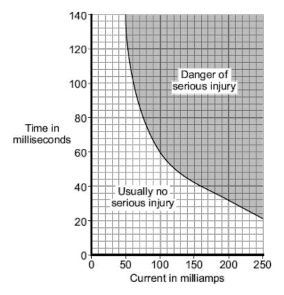
Using the RCCB helps prevent an electric shock seriously injuring the person using the hedge trimmers.
