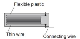
(a) (i) Using the correct symbols, **add** to the diagram to show how a battery, an ammeter and a voltmeter can be used to find the resistance of the strain gauge drawn above.
