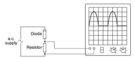
Why does the diode cause the trace on the oscilloscope screen to change?
