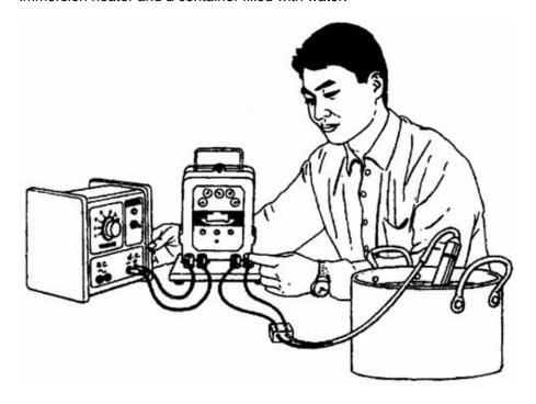
The voltage was set at 6 V d.c. The reading on the joulemeter at the start of the experiment was  $78\,882$  and 5 minutes later it was  $80\,142$ .
