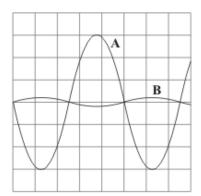
Trace  ${\bf A}$  shows how the potential difference between the live and neutral terminals of an electricity supply changes with time.
