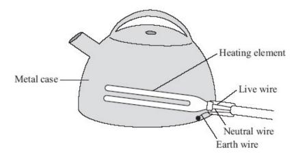
If a fault makes the metal case live, the earth wire and the fuse inside the plug protect anyone using the kettle from an electric shock.
