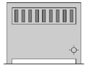
(i) A current of 11A flows when the fan heater is working normally. Fuses of value 3A, 5A, 10A and 13A are available. Which one should be used in the plug of the fan heater?
