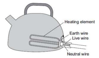
If a fault makes the metal case live, the earth wire and the fuse inside the plug protect anyone using the kettle from an electric shock.
