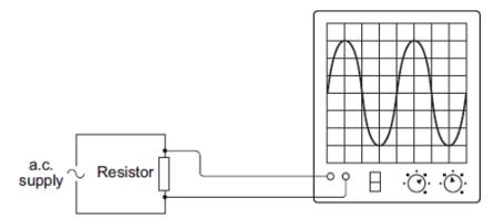
Each horizontal division on the oscilloscope screen represents a time of 0.01s.
