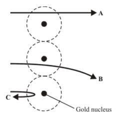
Explain the different paths A, B and C of the alpha particles.
