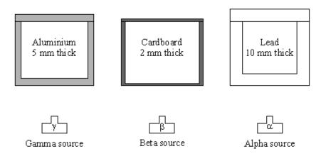
Draw lines to show which source should be stored in each box so that the risk of radiation leakage is a minimum.
