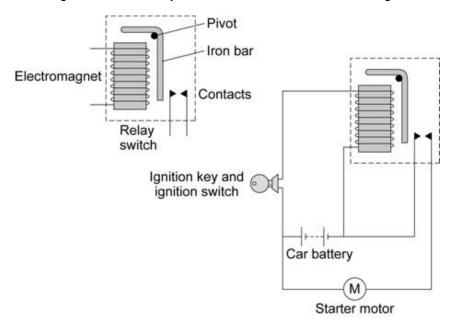
Turning the ignition key closes the ignition switch.
