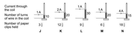
The student wants to find out how the strength of an electromagnet depends on the number of turns of wire in the coil.
