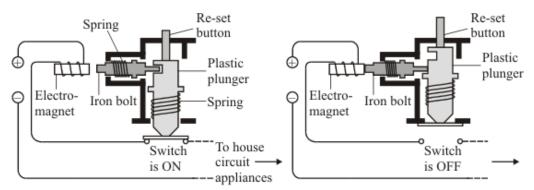
Describe, in as much detail as you can, how this circuit breaker works.
