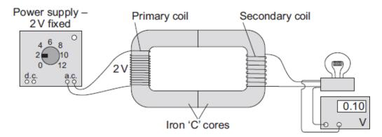
(a) The transformer made by the student would not have worked if the core had been made from aluminium and not iron.
