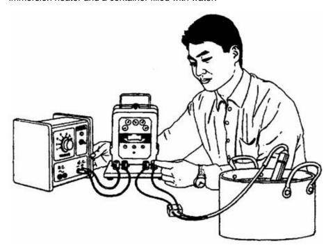
The immersion heater is designed for use in a tropical fish tank. It is connected to a step-down transformer supplied by 230 V a.c. mains.
