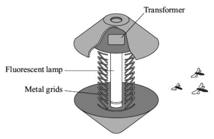
A transformer is used in the fly killer. There is a p.d. of 230 V across the primary coil. There are 300 turns of wire on the primary coil and 4000 turns on the secondary coil.
