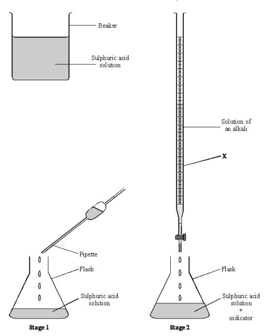
**Stage 1** 25.0 cm<sup>3</sup> of the sulphuric acid solution was added to a flask using a pipette.
