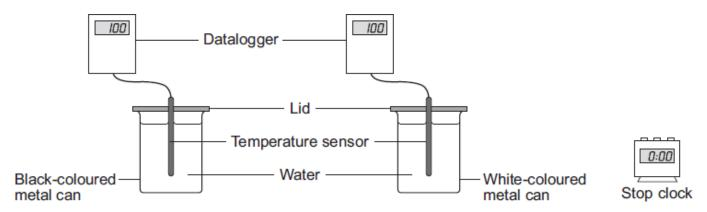
An equal volume of boiling water was poured into each metal can. The student then recorded the temperature of the water in each can every minute for ten minutes.
