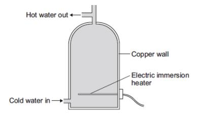
Energy is transferred by the process of convection from the hot water at the bottom of the
